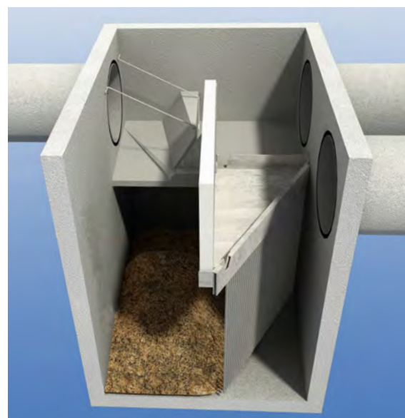
Figure 4 – Dual Outlet HumeGard® GPT
